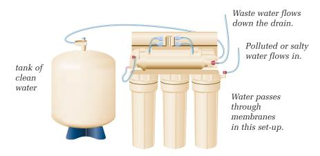
**Figure 1.9** This simple lab apparatus can create pure water.
