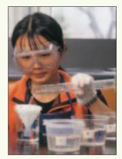
**Figure 1.6** Step 3. Pour 100 mL of one water sample through the filter.
