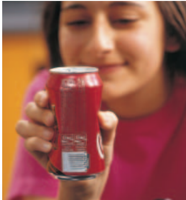
Figure 3.3 When you apply a very small force to an aluminum can, its sides start to dent, but will return to the original shape when the small force is released. If you apply a greater force, the dent may become permanent, and the can is deformed permanently.
