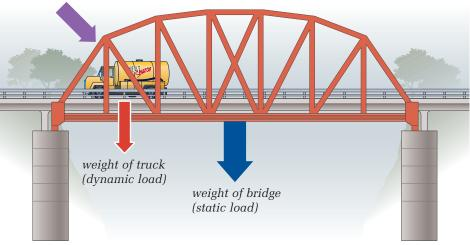
**Figure 2.13** Forces acting on this bridge include the weight of the bridge (static load), the weight of the truck (dynamic load), and the wind (dynamic load).
