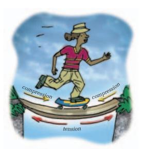
**Figure 2.26** Complementary forces—The weight of the girl results in compression and tension in the beam.
