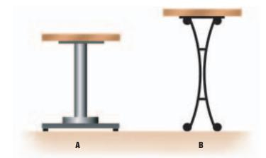
Figure 2.9 In most cases, structures with a low centre of gravity and wide base are stable. Which of these tables do you predict is the more stable of the two? Why do you think that?
