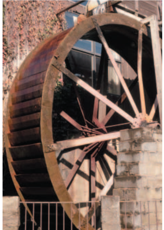
Figure 2.21 Flowing water causes this huge wheel to move. Linkages connect the moving wheel to mechanical systems that operate the mill.
