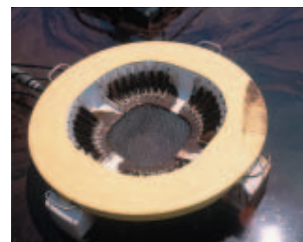
Figure 3.19 Oil floats on water, so clean-up crews can use skimmers such as this one to skim oil off the water's surface.
