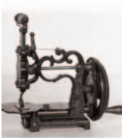
Figure 3.14a) Early sewing machines were operated by a hand crank. They could sew only simple stitches.
