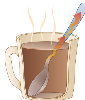
Figure 2.22 A metal spoon in a mug of hot chocolate. Heat is transferred from the hot liquid to the spoon. The particles in the spoon speed up and the spoon becomes hot.
