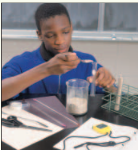
Figure 2.33a) Step 1. Filling the test tube with sand
