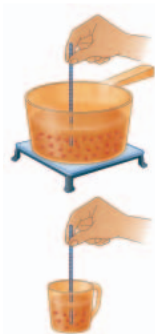
Figure 2.7 The soup in the pot has more thermal energy than the soup in the cup. But both are the same temperature.
