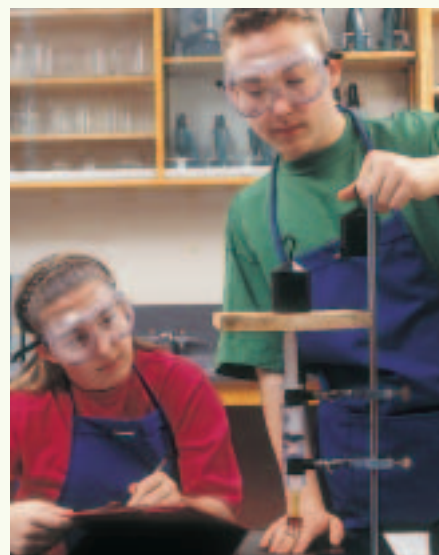
Figure 3.15 Step 7. Be sure to follow safe work procedures. Clamp the syringe tightly at right angles to the stand.
