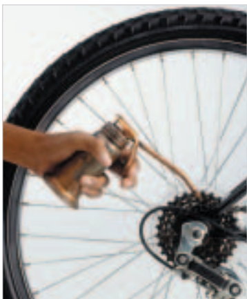
Figure 1.8 Your bicycle starts to make grinding noises as you pedal. What do you do? You use oil on your bicycle or in a car to make sure that the parts operate smoothly together. The viscosity of the oil that you use is important. Viscosity describes how easily a fluid flows. You will learn more about viscosity in section 3.0.
