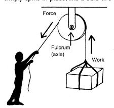
When a wheel has a groove on the outer edge and turns freely on an axle attached to a stationary position, you have a form of wheel and axle called a fixed pulley. This system uses rope wrapped over a wheel-and-axle system to change the direction force is applied (see Fig. 4). Gravity works for you, not against you.
