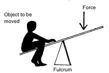
approaches. All levers consist of three parts: a part where you apply force, a fulcrum and a part where the object is moved (see Fig. I). The fulcrum provides a pivot point that changes the direction in which the force is exerted. By pushing down instead of lifting up, you take
