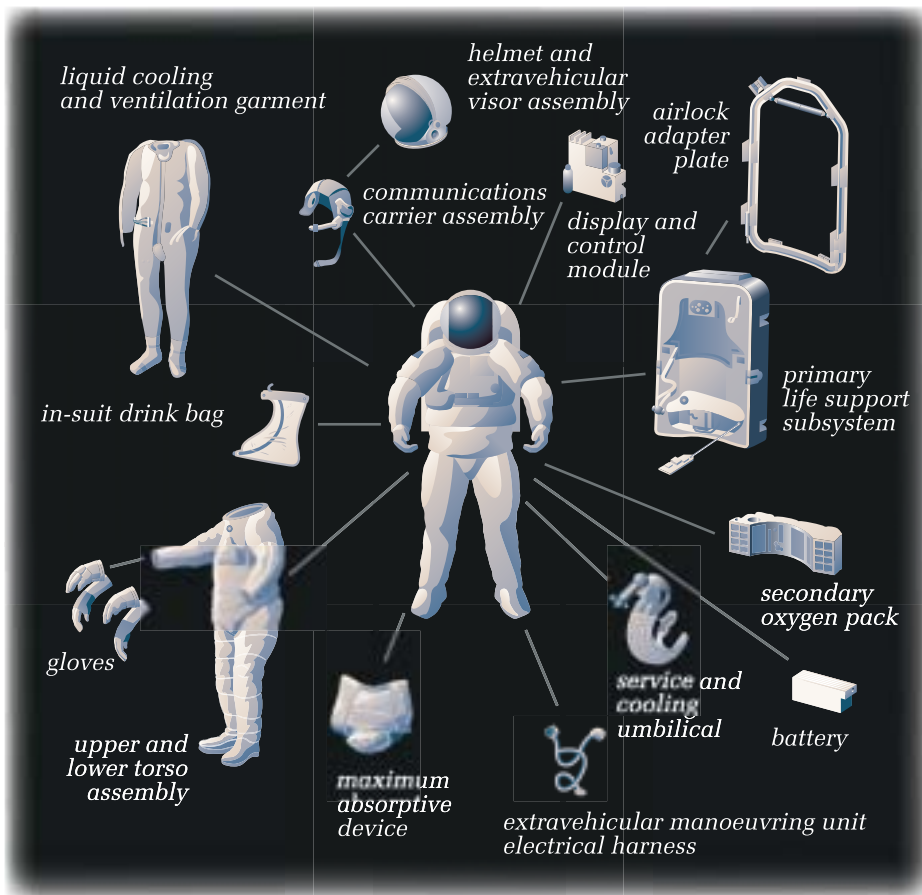
Figure 2.18 The first astronauts to walk in space were connected to their spacecraft with a hose that supplied oxygen and a means of communication. Modern astronauts use a suit that is completely self-contained, enabling them to work outside their crafts for up to 9 h at a time.
